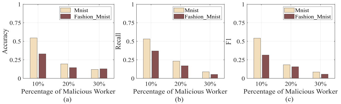
Fig. 6. (a) Accuracy, (b) Recall, and (c) F1 of global model under the different numbers of malicious participants.
