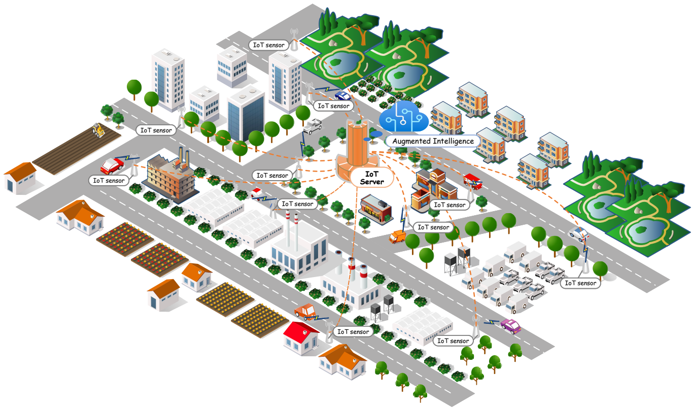
Fig. 1. Vehicle-road collaboration system applying AIoT. This is achieved by using wireless communication devices (e.g., sensors installed on the road) to collect vehicle trajectory information (e.g., average speed and flow rate of passing vehicles), after which the collected data is processed and analysed by augmented intelligence (e.g., deep learning or machine learning).
